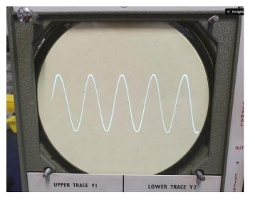
The CRT was manufactured in a manner where the Yellow Phosphor was applied to the glass faceplate of the CRT first and the Blue second. Looking at the inside of the CRT (which can be seen through the side wall of the tube) the internal appearance of the phosphor surface there is vivid Blue:
