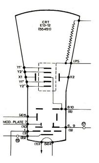
The CRT also has an IPS (Inter-plate shield) electrode to reduce the interactions of the two Y sets of plates. The service manual omitted advice on how to set the IPS voltage. It is usually set to the average deflection plate voltage which is 207V in the D52.
