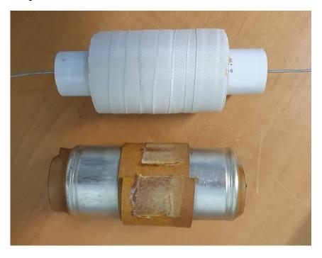
The photo below shows the two VMI rectifiers fitted and the two new capacitors in the voltage doubler:
