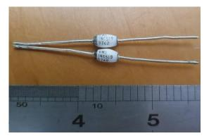
The new EHT rectifiers resulted in an increase in the EHT output from 2.6kV to 2.9kV or about a 11% increase in the final Anode voltage. The total CRT EHT voltage is higher though, because the CRT's cathode circuit is configured to run at -960V.
