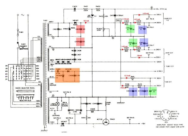
I went to a considerable amount of trouble to decide if C412, a 3 section 32uF 450v capacitor, shown in green above should be replaced. After removing it, extensive testing on its Capacity, Leakage at full rated voltage & ESR were all perfectly normal. So I re-fitted it. Also I could not find anything wrong with the main 120uF voltage doubler capacitors (shown in pink above) so they also got to remain as did most, but not all, of the other electrolytic capacitors in the scope.
